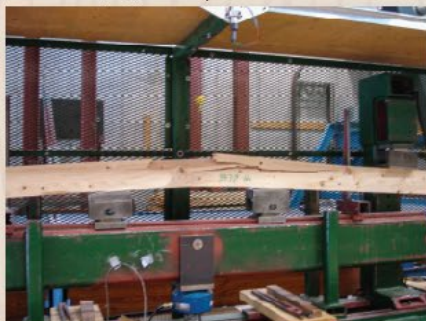
The development and maintenance of lumber design values for Canadian species includes testing of grade stamped lumber.
