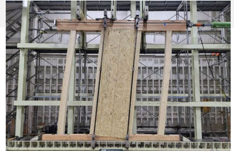
▲ Multi-year High Performance Shear Wall Testing for Midrise market
